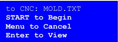
After pressing Start, the CNC will receive the data file selected. In the example above, file data contained in MOLD.TXT will be sent to the CNC. When the transmission is complete, the
