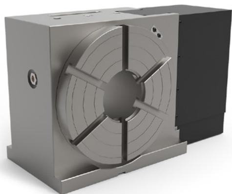
The VH-11 features a T-slot design to support the common 6 hole bolt circle found on most chucks. Using the standard spread allows ease of mounting a variety of chuck sizes and fixtures. The VH-11 is designed to be compact and rigid, using dual bearings for spindle and worm.
